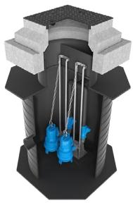
The Aquafix FLOWFIX plug and play pumping stations are designed for efficient removal of wastewater, stormwater and drainagewater. The body of these pumping stations is manufactured out of durable 1st. class new HDPE material. The pumping stations are standard equipped with a PE/PP telescopic manhole cover DN 600 or 800mm load class A. 15kN (EN 124). For a small surcharge you can opt for a cover class B. 125kN. or D. 400kN.
